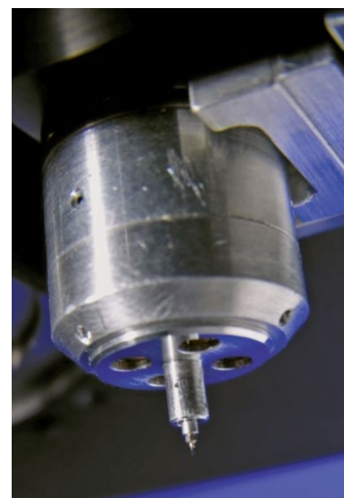
DCMII head with Berkovich tip installed
