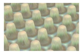
Fig.5. Measurement of PSS Bumps Using Zeta 20 3D Optical Profiler
