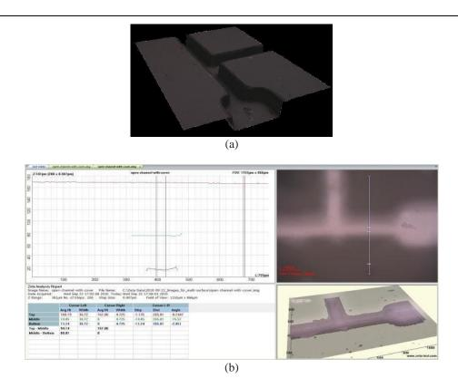
Fig.5 (a) 3D-mapping an open micro fluidics ,(b) 3D mapping a sealed micro fluidics cell
