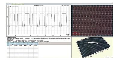
Fig.2.Measurement of PSS Bumps using AFM+Zeta Optical Profiler
