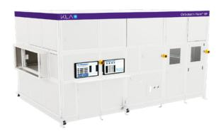
Orbotech Flare BP Inspection and Metrology System: Full inspection of the entire panel area enabled by WireSense™ innovative detection technology. This supports irregular and complex pixel design on both the front and back of the glass.
