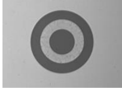
Figure 9. Circular patterns are rotationally symmetric, so are a poor choice for Geometric pattern recognition.
