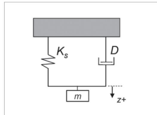
Figure 4. Dynamic model of instrument alone (no contact).
