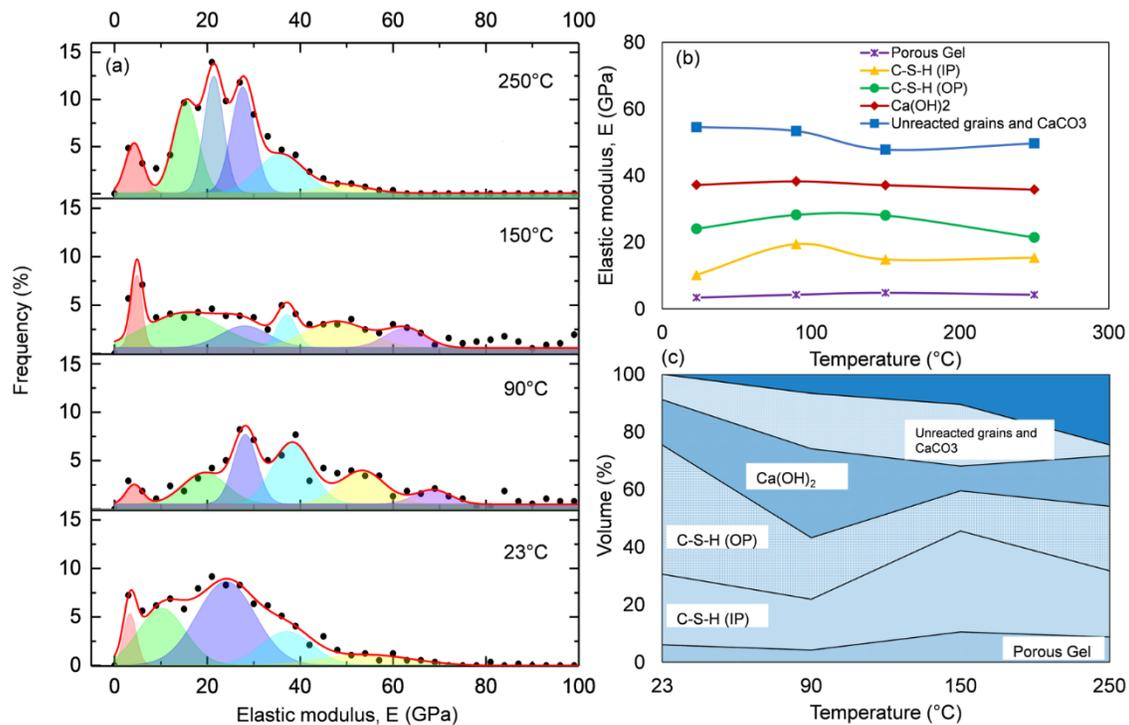
**Figure 3. (a) Frequency distribution of elastic modulus for OPC paste at different temperatures; (b) variation of elastic moduli of the microscopic phases with temperature; and (c) volume fractions of the microscopic phases as obtained from statistical nanoindentation analysis.**
