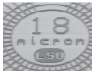
Fine lines / spaces of 18µm
