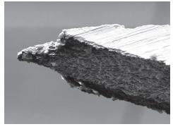
Chemically etched micro needle current industry level
