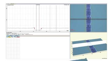
Figure 7: A laser induced trench in a thin film of Indium Tin Oxide (ITO) on a glass substrate used in flat panel displays. This laser-scribed trench is 8.6 μm in width and 0.2 μm in depth. >>
