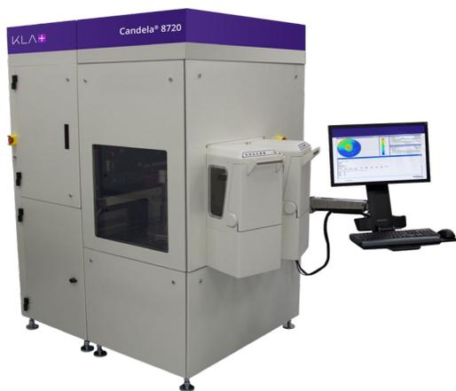
The Candela® 8720 advanced surface inspection system captures a variety of mission-critical substrate and epitaxial defects for the LED, photonics, communications and other compound semiconductor markets.
